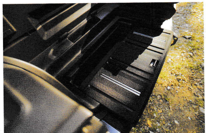
Part of the multi-function rear door of the Traveler is a shelf that pulls out when the lift gate is open – making it easier to sit in the back, protected from the rain, when tail-gating.
